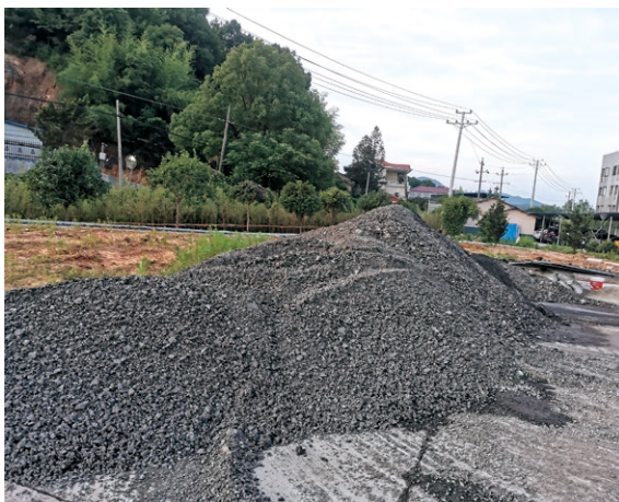
Collected waste bituminous for recycling
