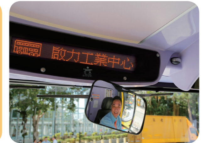
Automatic Bus Stop Announcement System on the bus fleet of NWFB and Citybus
