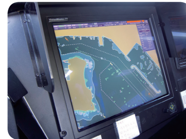
NWFF's Automatic Identification System presents the bearing and distance of nearby vessels equipped with the same system
