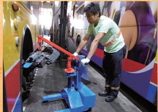
The "Workshop Popeye" lifting device, developed by bus depot employees, improves efficiency and enhances occupational safety.
