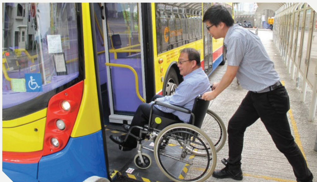
The entire bus fleets of NWFB and Citybus are designed to be barrier-free. Features such as low-floors and wheelchair ramps enhance accessibility.
