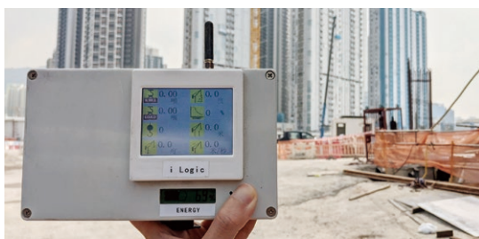
Wireless lifting monitoring system for tower cranes
